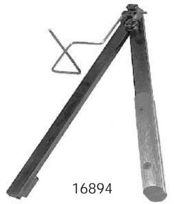
A tough tool that makes difficult wire repairs easy. You can bend the ends of no sags, edgewise and foam springs right on the spot, making offsets where you need them. Can be readily mounted in a vise for duplicating complex repetitive wire bends. Constructed of heat-hardened steel for long life.
