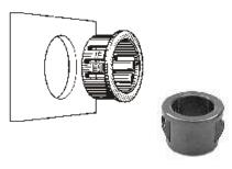
Nylon bushings designed to protect wires, cables, tubing, etc. from sharp, unfinished panel edges. Each size bushing employs multiple lock features to positively snap into panels ranging from 1/32" to 1/8" thickness. Available in both black and white nylon.
