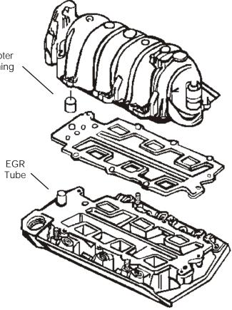
As an added benefit, the smaller diameter of our EGR port tube creates an air space between the repaired (with adapter bushing) upper plenum and the new EGR port tube. This air space insulates the composite material of the plenum from further damage.
