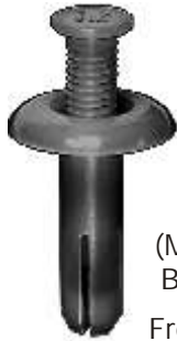
17472 (Mitsubishi: MB547806; Nissan: 63854-01A00) Black Nylon Front Bumper Fascia Push-Type Retainer Head Diameter: 20mm Stem Length: 20mm Fits Into 8mm Hole
