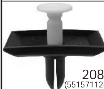
19638 (Chrys: 4805405AA; Ford: 1L5Z-17K826AA) Black & White Nylon Front Bumper Fascia Push-Type Retainer Head Dia.: 34mm Stem Length: 20mm Fits Into 8mm Hole Concorde, Intrepid, Eagle Pacifica & PT Cruiser 1998-On Ford Trucks 2005-On UNIT PACKAGE: 15
