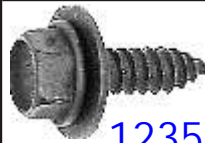
12351 (11505022) Black Polyseal Finish M6.3-1.81 x 20mm (#14 x 25/32") Hex Washer Head Sems® 17mm (11/16") Wshr O.D. 10mm Hex GM UNIT PACKAGE: 50
